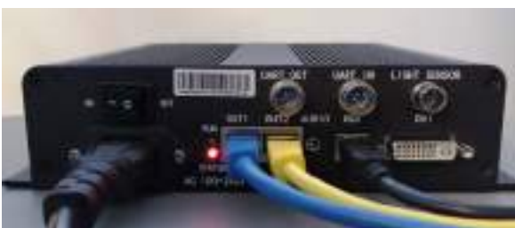
MCTRL300 controller with 2 data flows: Output 1 = flow 1 (blue), output 2 = flow 2 (yellow)
