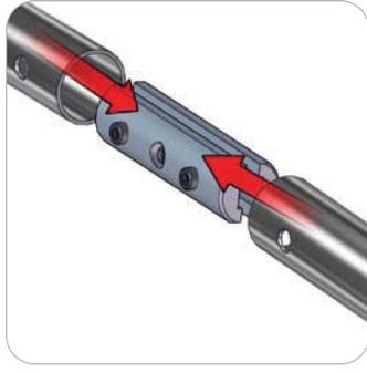
Compress the unlocked connector and slide one tube onto each end. Lock both screws carefully using your allen key tool. Be sure to lock securely, but do not overtighten.
