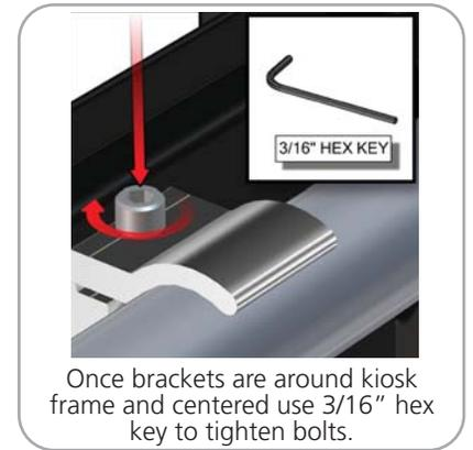
Once brackets are around the kiosk frame and centered use 3/16" hex key to tighten bolts.
