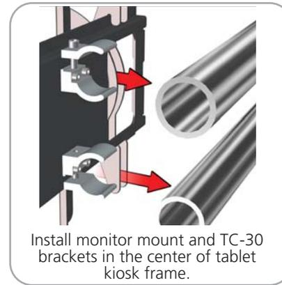
Install monitor mount and TC-30 brackets in the center of tablet kiosk frame.
