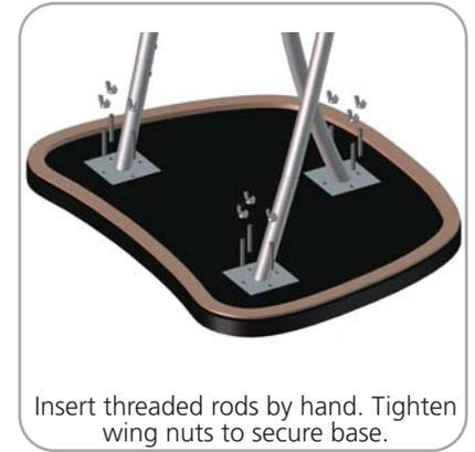
Insert threaded rods by hand. Tighten wing nuts to secure base.
