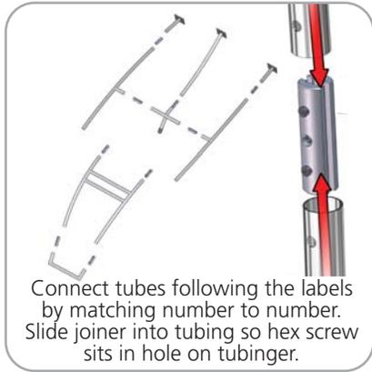
Connect tubes following the labels by matching number to number. Slide joiner into tubing so hex screw sits in hole on tubing.
