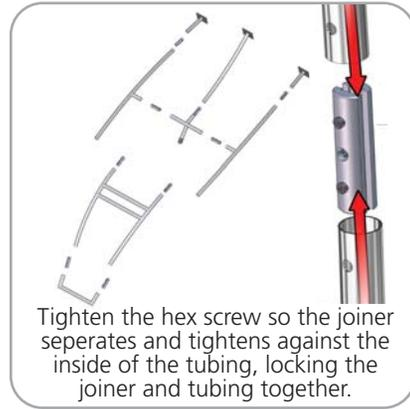
Tighten the hex screw so the joiner separates and tightens against the inside of the tubing, locking the joiner and tubing together.
